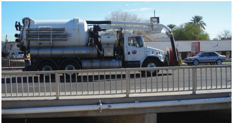
Two city of Phoenix loaded water trucks were used for the static load testing. These trucks had a three-axle configuration with a gross vehicle weight of 60 kips.
